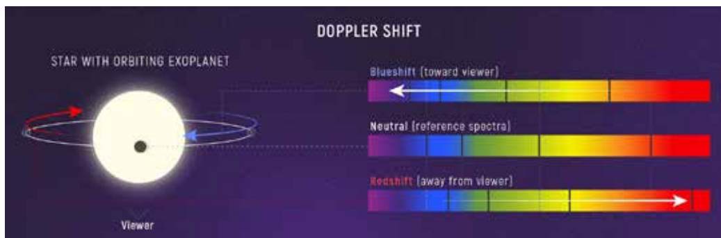
As a planet orbits a star, the star wobbles. This causes a change in the appearance of the star's spectrum called Doppler shift. Because the change in wavelength is directly related to relative speed, astronomers can use Doppler shift to calculate exactly how fast an object is moving toward or away from us. Astronomers can also track the Doppler shift of a star over time to estimate the mass of the planet orbiting it. Credit: NASA, ESA, CSA, Leah Hustak (STScI)
